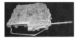
2. Remove Lo/Overrun check ball from valve body as pictured, this cavity will remain empty. Note location of (2) remaining check balls, they will remain in the same location when valve body is re-installed. The check ball that is removed will be used later.
