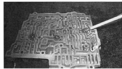
3. Remove the Overrun clutch valve assembly as pictured. Re-install in reverse order with the check ball removed in step (2) being installed first. The valve face touching the check ball may need to be ground for clearance.
