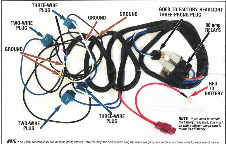
NUTE - All 4 blue ceramic plugs are the three-prong version. However, only one blue ceramic plug has two wires going to it and one has three wires for each side of the car. It's important that the two-wire ceramic plug goes to the (inner) high beam headlight and the three-wire plug goes to the (outer) low beam headlight. All the new H4 headlight bulbs are three prong, which is the reason why the plugs are all three prong.
