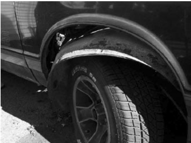
Step 2: Now remove the right front (passenger side) plastic inner fender to allow access to the firewall area.
