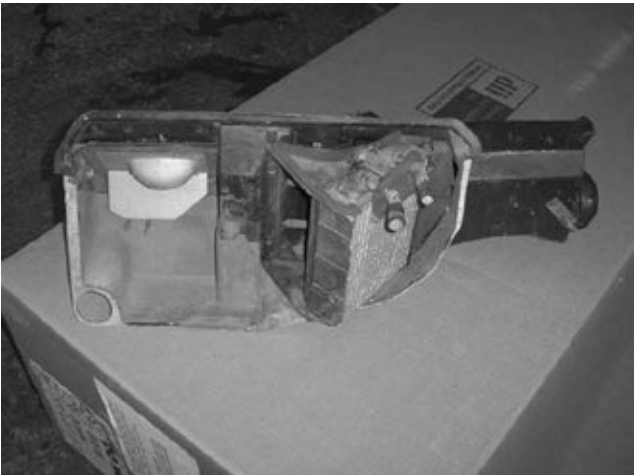
Step 14: Reassemble the piece that was cut from the evaporator unit to the under dash duct work as shown. Including the heater core.
