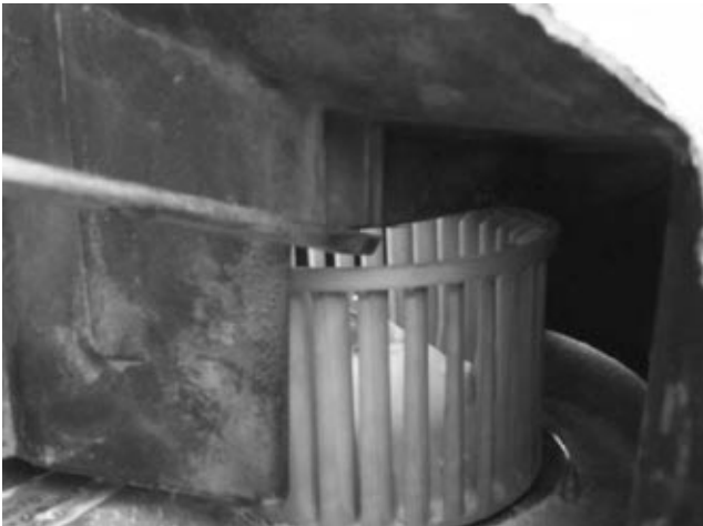
Step 22: Attach your blower motor and fan to the new AC Delete cover and trial fit the modified blower housing as shown above. Make sure you have clearance for the blower fan to spin freely.
