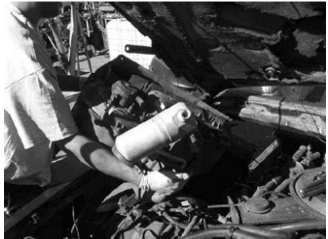
Step 5: With the hood hinge removed the AC unit should slide out in one piece revealing the large hole left in the firewall.
