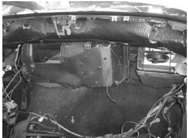
Step 3: This shows the under dash duct work that is attached to the evaporator cover under the hood. Remove all hardware that attaches the complete unit to the firewall.
