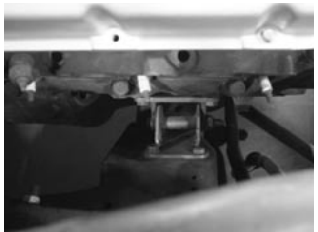
As an alternate, solid motor mounts can also be used, and are available from Moroso. (These are designed for racing applications).
