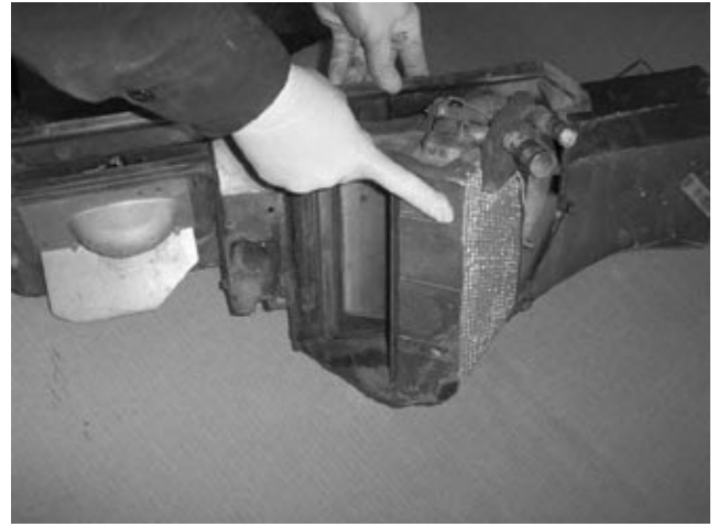
Step 13: You must trim the outer edge of the original heater core housing to allow proper clearance of the new AC Delete Cover. If this is not done the new cover will not fit!
