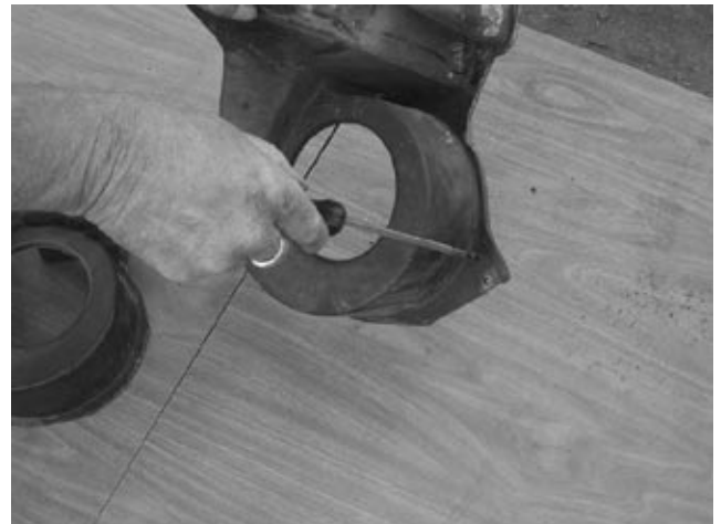
Step 17: Trim the housing in the area indicated above, to allow the housing to fit properly inside the new AC Delete Cover.
