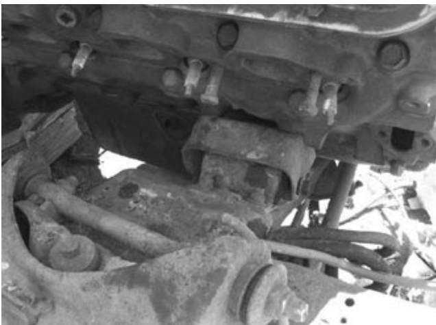
The stock GM motor mounts (shown above) are suggested as the best stock style application that you can use. Provided you use the stock motor mounts, clearance on any application is not a problem.
