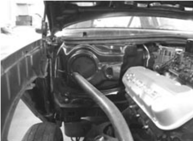
The photo above shows the AC Delete cover installed on an 81 Monte Carlo with a 454 big block and tall GM aluminum valve covers. As shown, there are no clearance issues for this application.
