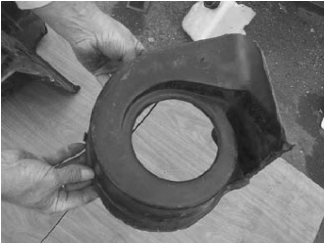
Step 20: Here is a close up topside view of the modified original blower motor housing. Your finished product should look just like this.
