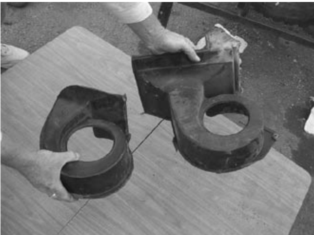
Step 16: Redesign the original blower motor housing as shown on the left to provide proper air flow to the heater core. This will allow your heater and defroster to remain functional. The part on the right is the original housing before modification.
