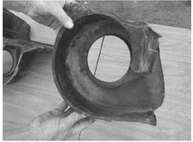
Step 19: Here is a close up backside view of the modified original blower motor housing. Your finished product should look just like this.
