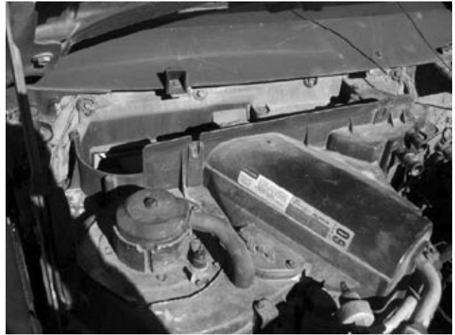
Step 1: Begin by removing the cowl screen and related pieces to provide access to the firewall mounting hardware.
