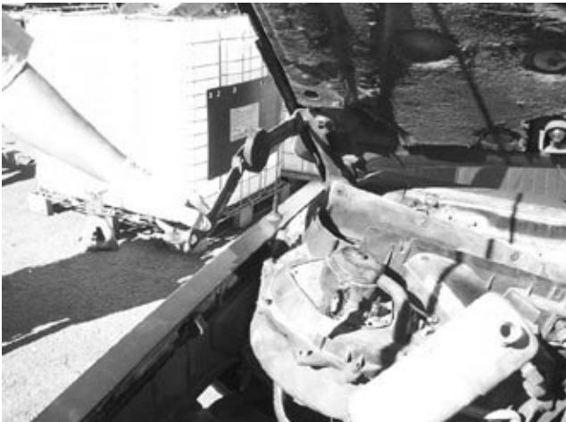
Step 4: Now you will need to remove the passenger side hood hinge to allow the complete AC unit to be removed in one piece.
