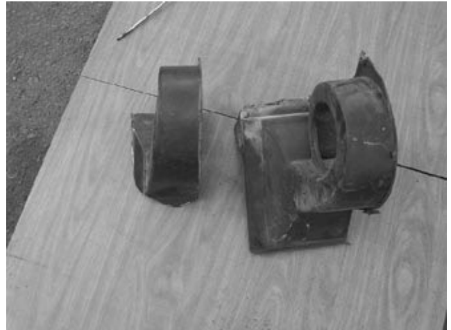
Step 21: Here is a close up side view of the modified original blower motor housing (left) compared to the original (right). Your finished product should look just like this.
